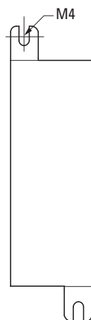
Figure 10: EU5C-SWD-CAN screw fixing
