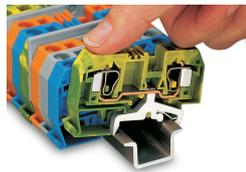
Snapping a ground conductor block onto the DIN-rail automatically makes a direct electrical connection to the rail.
