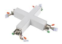
• X-shape connection unit for opal diffuser version of Otao Linear range, RAL9003 (white) finishing, direct distribution, only 3000K/4000K LED light sources included, feed by next straight luminaire, shipped with 4x fast connectors and additional replacement electrical connectors, 50mm wide extruded aluminium profile, nominal size: 290x290x50x73mm.
