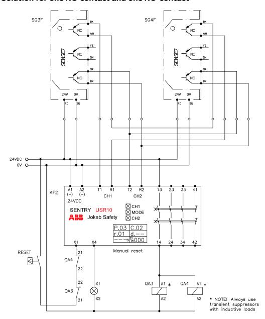
Note: The PL should be calculated using ISO/TR 24119 and EN ISO 13849-1/2
