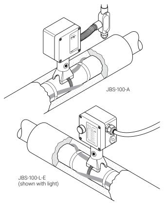
The nVent RAYCHEM JBS-100 kit is designed to connect power to a single nVent RAYCHEM BTV, QTVR, XTV, KTV, HTV or VPL industrial parallel heating cable. It is approved by FM, CSA, and PTB for use in hazardous locations.
