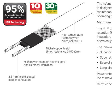
The nVent RAYCHEM HTV self-regulating heating cable is designed for freeze protection or process temperature maintenance of pipes and vessels with very high continuous operating temperatures (205°C).
