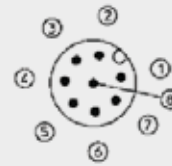
M12 8-pole (power supply and I/O)
