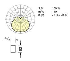
Furniture luminaire/mirror luminaire; Housing made of anodised extruded aluminium profile, screw fixable end faces made of plastic coated white aluminium (RAL 9006), vertical or horizontal wall mounting possible, with integrated cable duct and protection rated cable entry. Housing colour aluminium natural anodized; Direct/indirect light distribution using opal diffuser made of polycarbonate with smooth surface; Electrical connection via 3-pole connection terminal with plug-in contacts.
