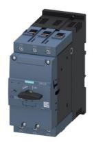
Circuit breaker size S3 for starter combination Rated current 84 A Nrelease 1170 A screw terminal Standard switching capacity
