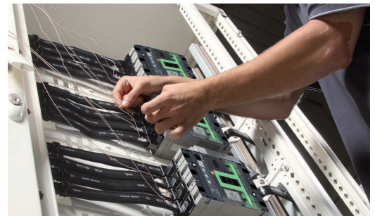
Temperature rise test in laboratory.
