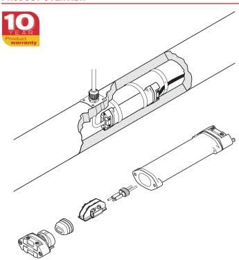
The nVent RAYCHEM C-150-E is a cold applied low profile power connection. The kit enables in line connection of nVent RAYCHEM industrial heating cables, BTV, QTVR and XTVR, to a flexible power cable. It can be used in applications with temperature ratings from  $-55^{\circ}$ C to 200°C. It is approved for use in hazardous areas.
