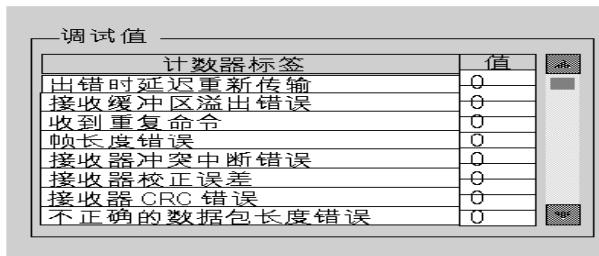
The screenshot shows a table titled '调试值' (Debug Values) with 10 rows, each representing a fault counter. The columns are '计数器标签' (Counter Label) and '值' (Value). All values are currently 0. The table has a light gray background and a dark gray header row. The labels in the first column are: '出错时延时重新传输', '接收缓冲区溢出错误', '收到重复命令', '帧长度错误', '接收器冲突中断错误', '接收器校正误差', '接收器CRC错误', and '不正确的数据包长度错误'.
