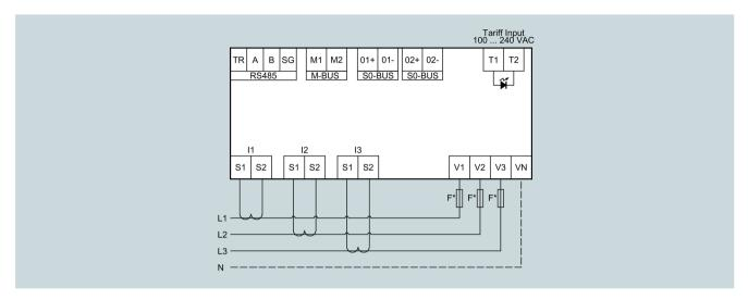
\* The fuse in the voltage measuring input is only used for cable protection.
