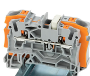
Step-down jumper (2006-499) commons 6/4 mm 2 (10/12 AWG) terminal blocks (2206/2204 Series) with 4/2.5/1.5 mm 2 (AWG 12/14/16) terminal blocks (2204/2202/2201 Series).
