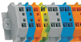
Terminal strip with mounting flanges, for screw or similar mounting types, 3.2 mm mounting hole diameter (with 209-123 Mounting Foot also for DIN-35 rail)
