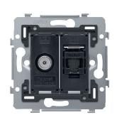
directions: If the flush-mounting box sticks out of the plasterwork, the multi-positional snap hooks can compensate for a 1 to 1.2 mm margin; if the flush-mounting box is sunk too deeply in the plasterwork, the snap hooks can compensate for up to a 1.8 mm margin. The end borders also have 4 round openings that ensure the correct positioning of the faceplate in relation to the central plate.
