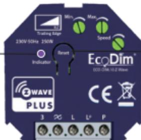
**Step 1.** Press the reset button for 3 times.
