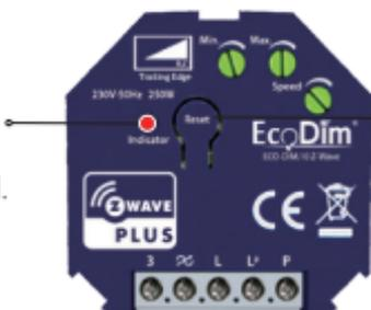
**Step 1.** Press the reset button for 5s.
