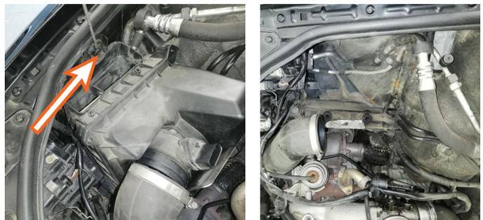
Pry out and remove the air filter by loosening the locking pin.<sup>4)</sup>
