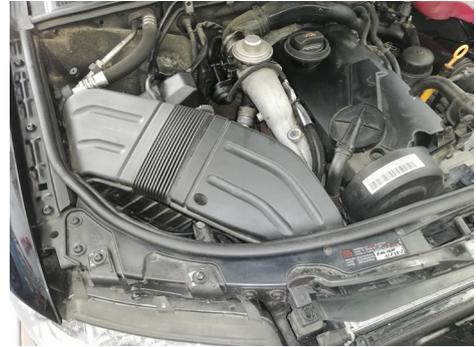
Detach and remove air intake duct.<sup>2)</sup>
