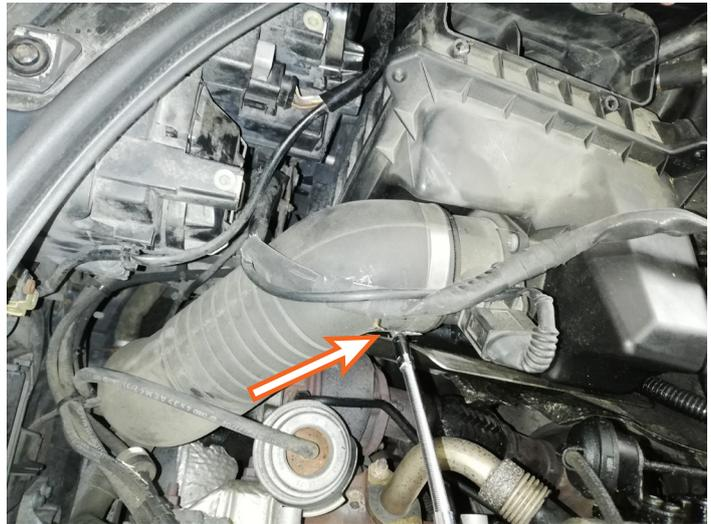
Pull hose from air filter by loosening the clamp.<sup>3)</sup>
