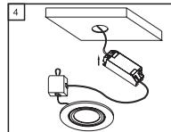
**Step 4 -** Connect the spots in series via the distribution box. Connect the loops to the empty connectors.
