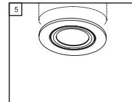
**Step 5 -** When properly installed, the recessed spotlight will clamp against the ceiling/ frame.
