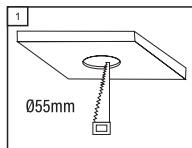
**Step 1 -** Cut a hole in the ceiling with a diameter of 55mm.
