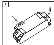
**Step 4 - Choose the light colour of the recessed spot using the slider.**
