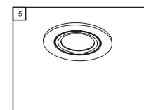
**Step 5 - If the recessed spot is positioned correctly, it will clamp against the ceiling.**
