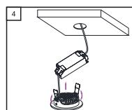
**Step 4 - Push the mounting clamps through the cut hole.**
