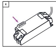
**Step 4 -** Choose the light colour of the recessed spot using the slider.
