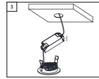
**Step 3 -** Connect the phase and neutral wire to the L and N side of the driver (indicated on the driver / transformer).
