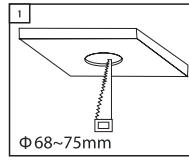
**Step 1 -** Cut a hole in the ceiling with a diameter of 68~75mm.
