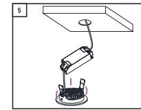
**Step 5 -** Push the mounting clamps through the cut hole.
