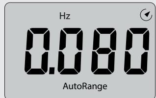
12. Press the Hz% button until "%" is indicate to read the % duty cycle in the display
