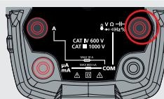
4. Touch the black test probe tip to the negative side of the circuit
