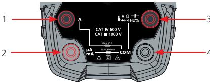
All functions except current use the VOHMS and COM input terminals. The two current input terminals.
