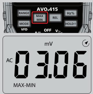
5. To exit MAX/MIN mode press and hold the MAX/MIN key for 2 seconds
