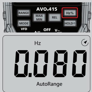
9. Press the Hz% button until "%" is indicate to read the % duty cycle in the display
