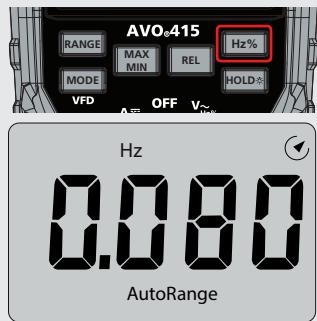
11. Press the Hz% button until "%" is indicate to read the % duty cycle in the display
