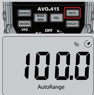
12. Press the Hz% button to return to the measurement
