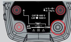
3. Insert the red test lead 4 mm plug into the  $\Omega$  terminal
