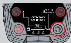
3. Insert the red test lead 4 mm plug into the Hz% terminal
