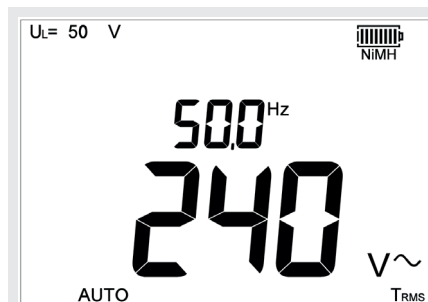
Figure 9: Instrument displaying that the circuit is live.
