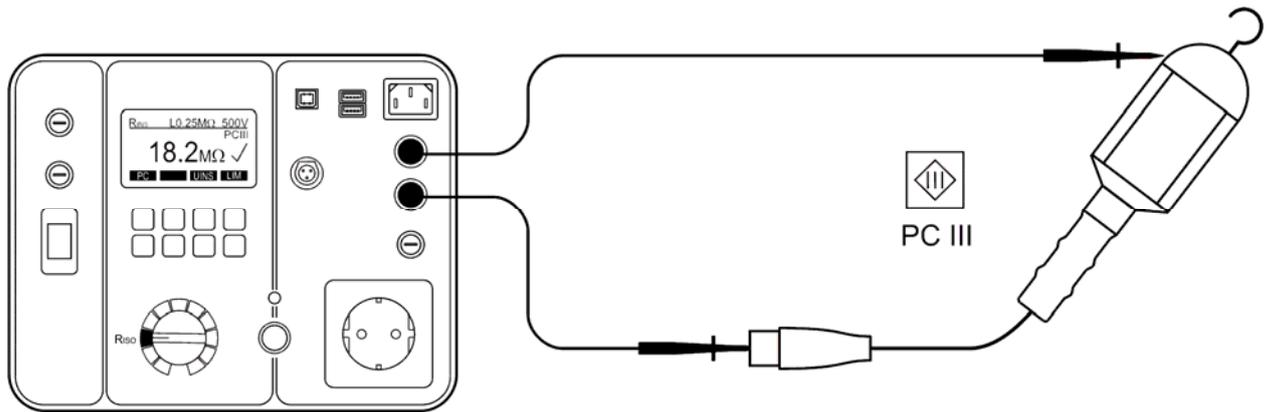
Figure 15: Insulation resistance test connections at appliance PC III. Use probe 1 and 2.
