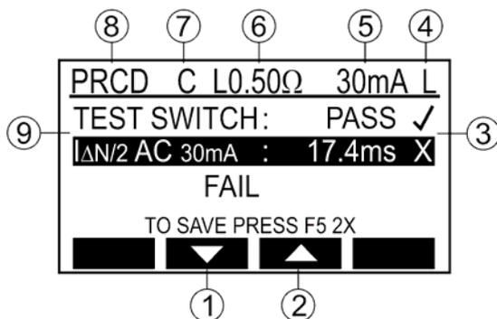
Figure 41: Display with test result in PRCD test (example)
