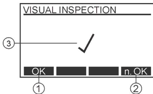
Figure 8: Display in visual inspection function (example)
