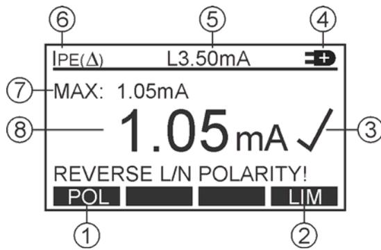
Figure 21: Display in earth leakage current test IPE (example)
