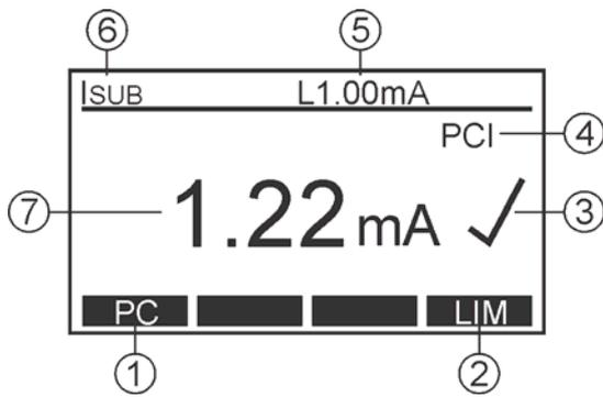
Figure 19: Display in substitute leakage current test ISUB (example)
