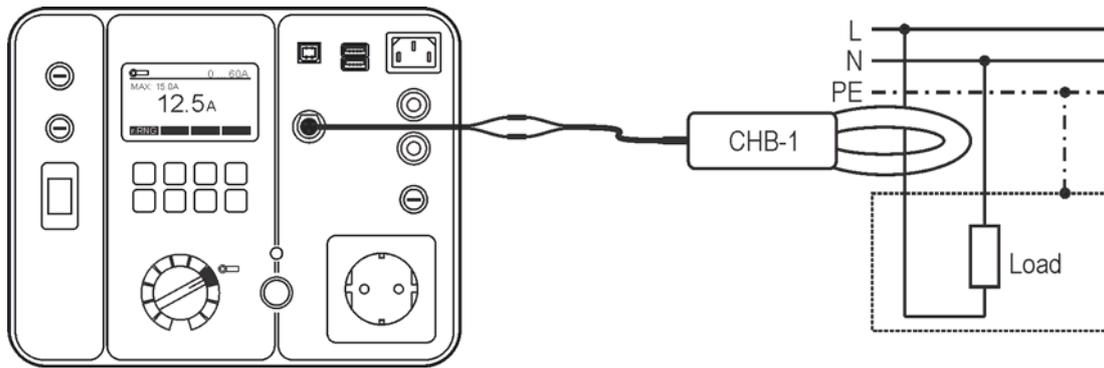
Figure 29: Load current test connection
