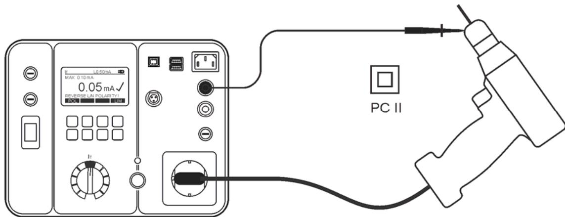
Figure 23: Touch leakage current test connections at appliance PC II. Use probe 2.
