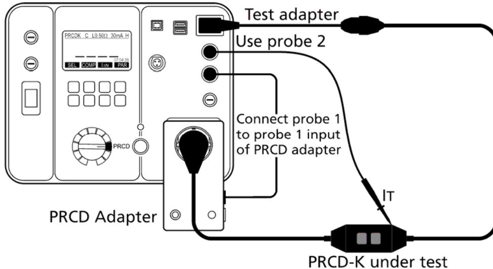
Figure 40: PRCD-K test connection
