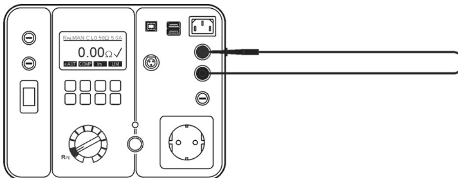
Figure 7: Connection for test lead compensation
