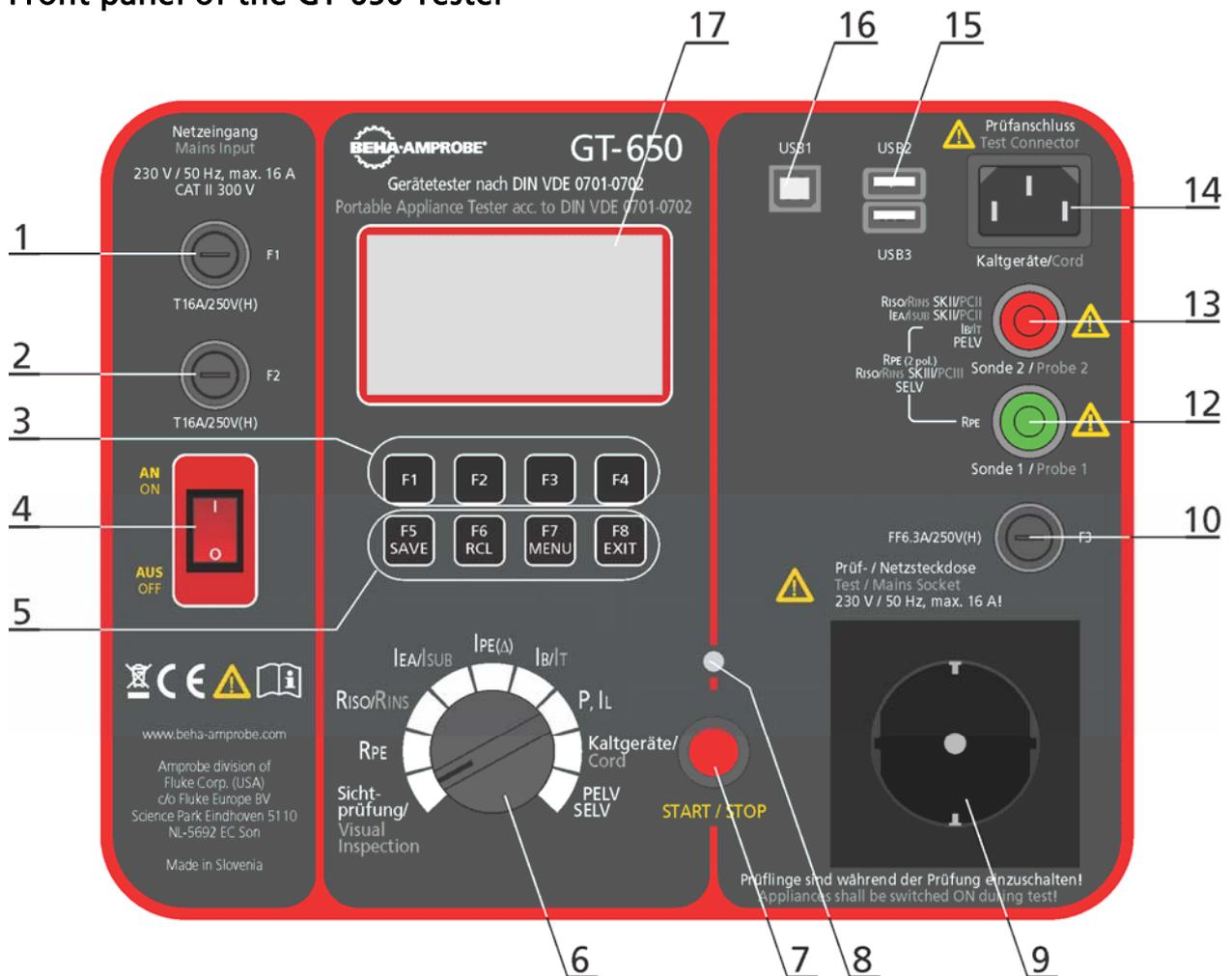
Figure 2: Operational elements and connectors on GT-650 tester
