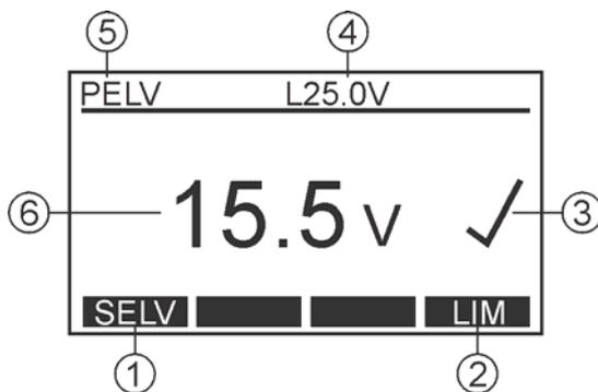
Figure 43: Display in PELV test (example)
