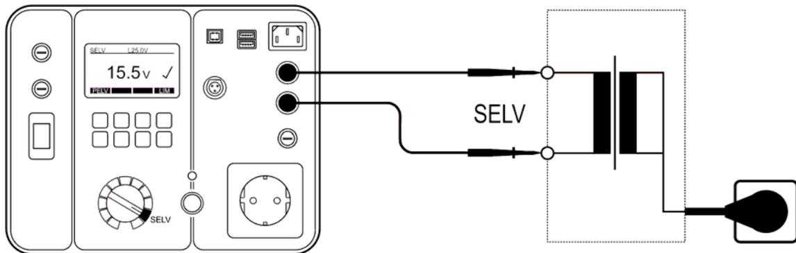
Figure 44: SELV test connection
