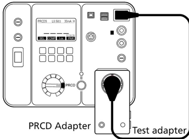
Figure 36: Connection of the PRCD Adapter for compensation purpose
