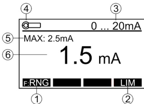
Figure 30: Display in CLAMP current test (🔋) (example)
