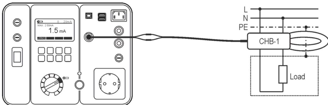
Figure 28: Earth leakage current test connection (direct method)
