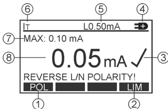
Figure 24: Display in touch leakage current test  $I_T$  (example)
