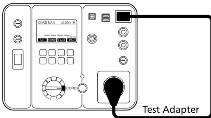
Figure 33: Connection of the Test Adapter for compensation purpose
