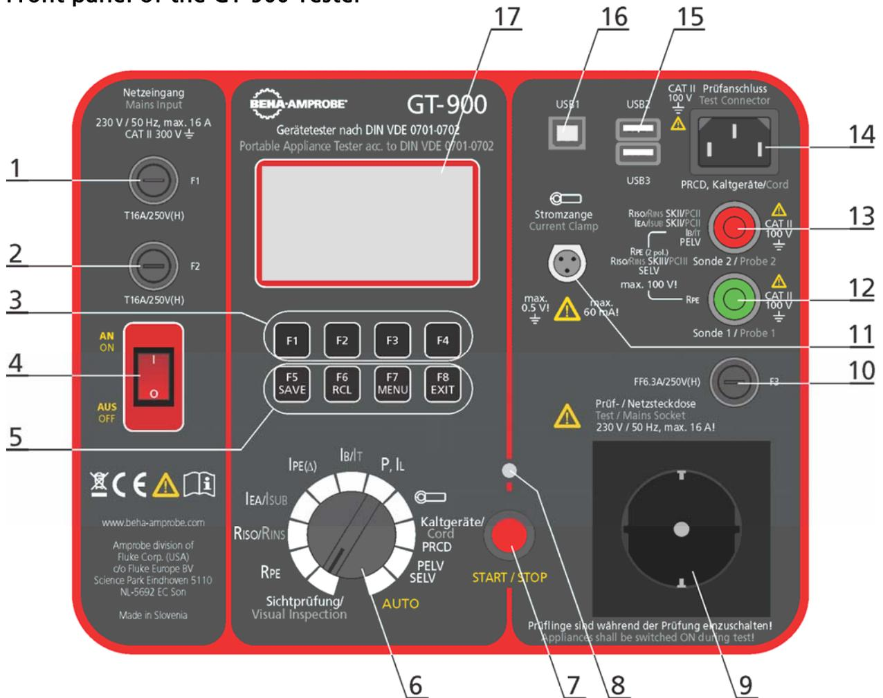
Figure 3: Operational elements and connectors on GT-900 tester
