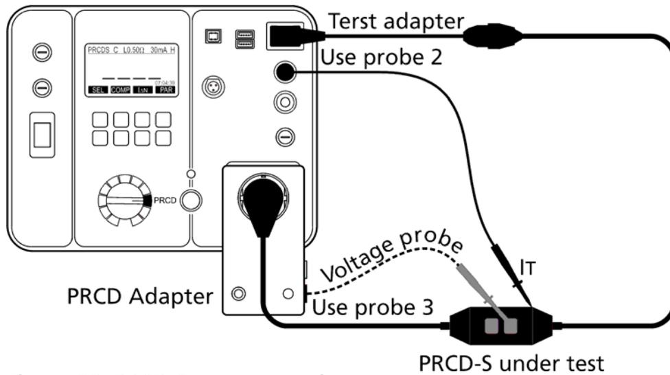
Figure 38: PRCD-S test connection
