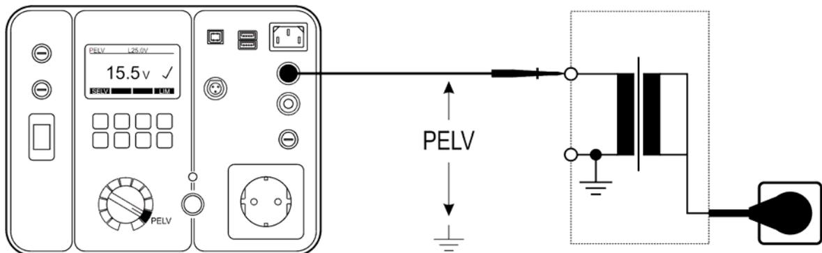
Figure 42: PELV test connection
