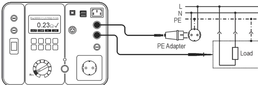
Figure 10: Protective earth bond test connections at permanently connected appliance. Use probe 1 and 2
