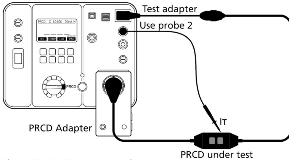
Figure 37: PRCD test connection
