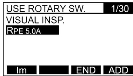
Figure 54: Test step selection menu (example, rotary switch is in RPE position)
