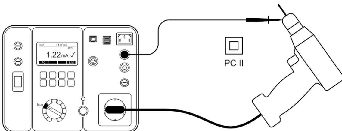
Figure 18: Substitute leakage current test connections at appliance PC II. Use probe 2.
