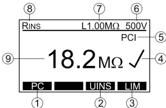
Figure 16: Display in insulation resistance test RINS (example)
