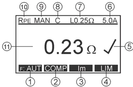
Figure 11: Display in protective earth bond test RPE (example)
