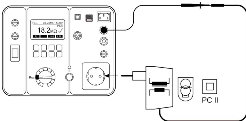
Figure 14: Insulation resistance test connections for power supply (PC II). Use probe 2.
