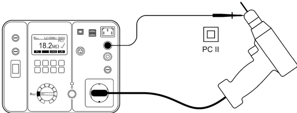
Figure 13: Insulation resistance test connections at appliance PC II. Use probe 2.
