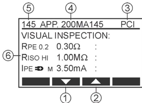
Figure 48: AUTO-TEST display after pressing the START key (example, TC# 145 was selected as an attribute to the appliance code)
