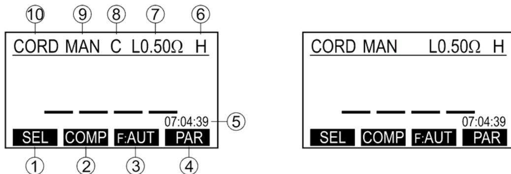
Figure 32: Idle display in CORD test (example), left picture - test adapter compensated (C present), right picture – test adapter not compensated (C not present)
