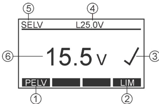
Figure 45: Display in SELV test (example)
