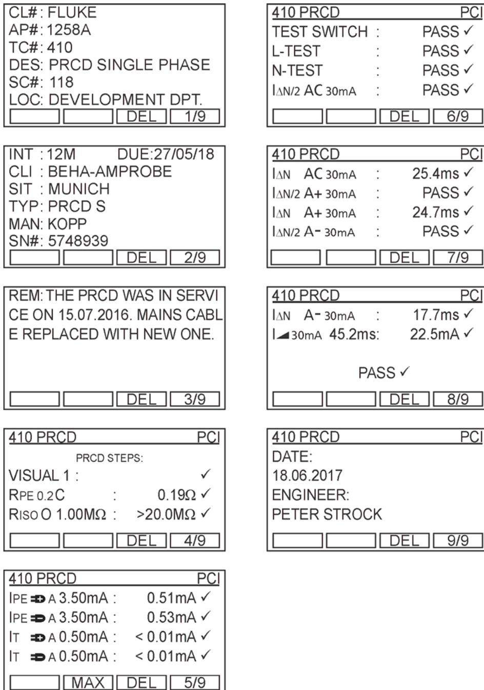
Figure 61: Recalled result (example for PRCD)
