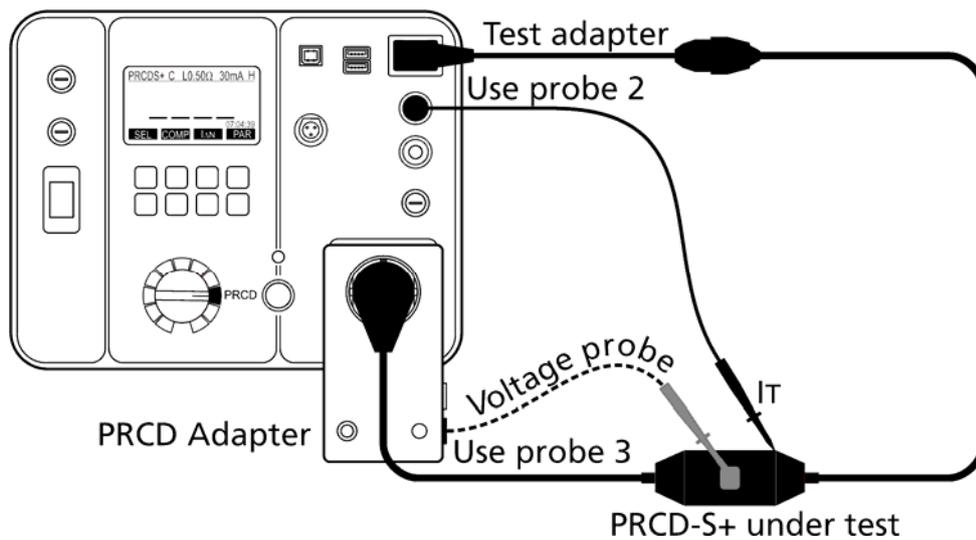
Figure 39: PRCD-S+ test connection
