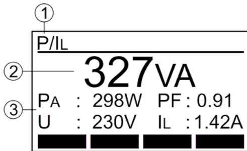
Figure 26: Display for Functional test P/IL (example)
