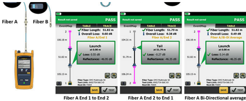
OptiFiber Pro's SmartLoop technology tests two fibers in one test while providing individual pass, fail and bi-directionally averaged results for each fiber link.
