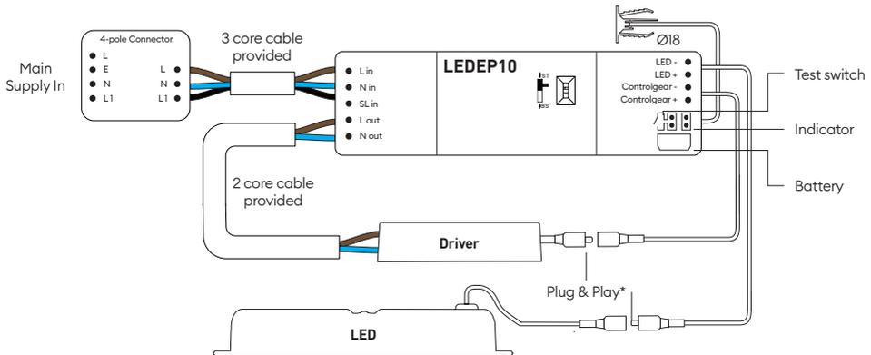
\* Make sure plug & play connectors polarity matches the products you are installing
