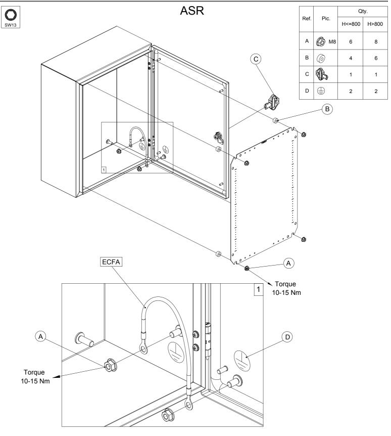
**WARNING:** When mounting on or over a combustible surface, a floor plate of at least 1.43 mm galvanized or 1.6 mm uncoated steel extended at least 150 mm beyond the equipment on all sides must be installed.
