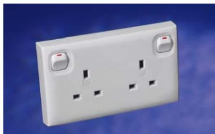
Bakelite resin twin switched 13A BS1363 socket outlet intended for mounting on recessed 1 gang boxes to convert 1 gang socket outlet to 2 gang socket without modification to existing wiring or building structure.
