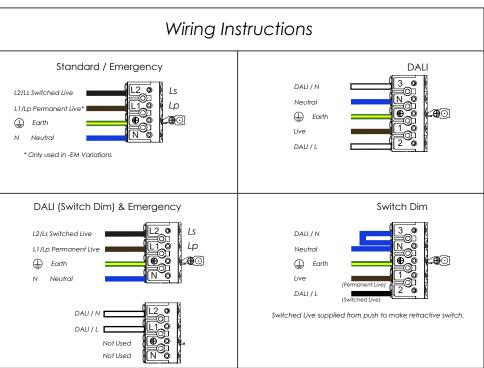
For Switch Dim wiring, connect a permanent live to L1 and wire supply from retractive switch (push to make) to DALI / L. Also link between N and DALI / N.
