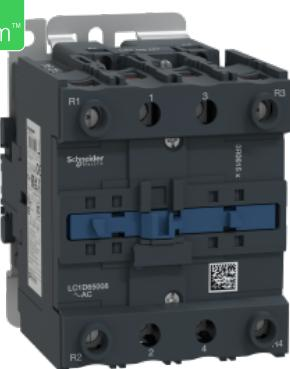
**TeSys D contactor - 4P(2 NO + 2 NC) - AC-1 <= 440 V 80 A 110 V AC 50/60 Hz coil**
