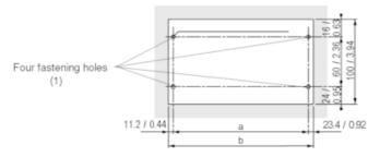
(1) The diameter of the fastening holes must allow use of M4, M5, M6 and UNC #6 screws.
