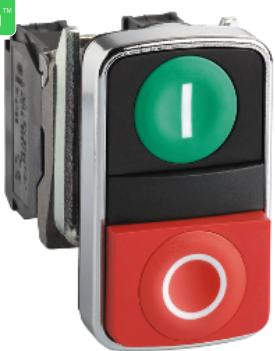
Double-headed push button, metal, Ø22, 1 green flush marked I + 1 red projecting marked O, 1 NO + 1 NC
