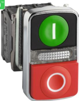
**Illuminated double-headed push button, metal, Ø22, 1 green flush I + 1 pilot light + 1 red projecting O, 1 NO + 1 NC**
