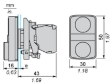
**Panel Cut-out for Pushbuttons, Switches and Pilot Lights (Finished Holes, Ready for Installation)**
