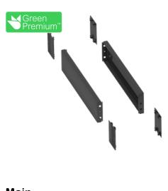
2 side panels for plinth. 400x100mm. Folded sheet steel. RAL 7022. IP 30. IK 10.
