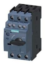
Circuit breaker size S00 for motor protection, CLASS 10 A-release 5.5...8 A N-release 104 A screw terminal Standard switching capacity with transverse auxiliary switches 1 NO+1 NC
