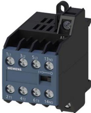
Power relay, AC-3 8.4 A, 4 kW / 400 V 4 NO, 230 V AC, 45...450 Hz 3 pole, screw terminal
