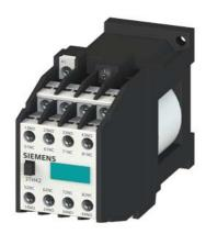
Contactor relay, 44E, DIN EN 50011, 4NO + 4NC, screw terminal DC operation 125 V DC
