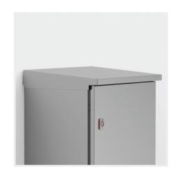
**Description:** To be fitted as an outdoor shelter on stainless steel wall mounted enclosures. The roof is slightly sloped and has a drip strip. Machining is required. Dimensions of the enclosure will be increased by H: 60 mm, W: 20 mm and D: 20 mm.
