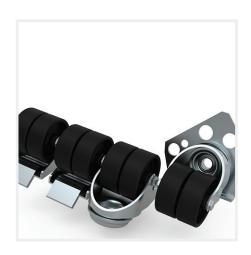
**Description:** For easy transportation of an (equipped) enclosure. Can be mounted directly to the enclosure's frame or underneath the plinths (PF/PV) with the provided mounting brackets. Raises the enclosure by 70 mm.
