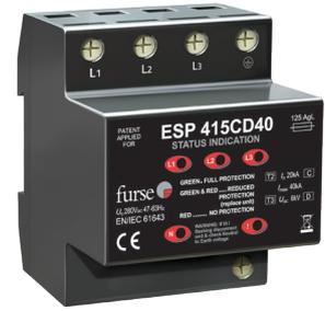
Compact combined Type 2 and 3 tested (to BS EN 61643) Surge Protective Device (SPD) for use on three phase mains power distribution systems primarily to protect connected electronic equipment from transient overvoltages on the mains supply, e.g. computer, communications or control equipment. For use at boundaries up to LPZ 1 through to LPZ 3 to protect sensitive electronic equipment.
