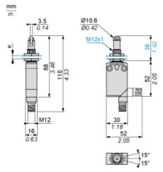
e: 8 mm max, panel cut-out Ø 12.5 mm, fixing nut thickness 3.5 mm.
