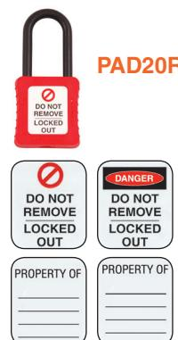
Plastic body padlock with 6mm hardened insulated shackle. Designed for use with Martindale lock out devices and compatible with most other safety lock out products. Padlock body width - 38mm. Vertical shackle clearance - 38mm.
