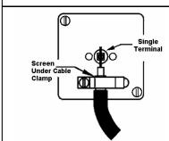
Each coaxial cable should be connected to the appropriate terminal as shown.
