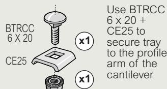
Use BTRCC 6 x 20 + CE25 to secure tray to the profile arm of the cantilever
