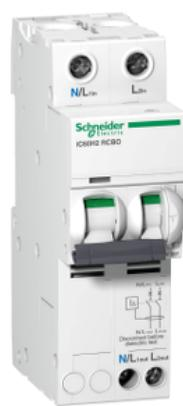
**iC60H2 - earth leakage circuit breaker - 2P - C curve - 32 A - 30 mA - 110 V**
