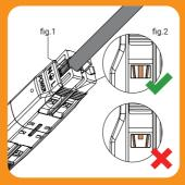
Check there is a sufficient length of outer cable sheath available for clamping. (fig.1) and that an unbroken length of conductor occupies the full extent of the window (fig.2).
