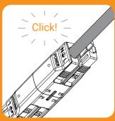
Push cable until it snaps into place. Repeat process for additional cables. Push in any unused cable entries.
