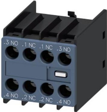
auxiliary switch, on the front, 2 NO + 2 NC, .3/.4, .1/.2, .1/.2, .3/.4, current path: 1 NO, 1 NC, 1 NC, 1 NO, screw terminal, for contactors 3RT2 and contactor relays 3RH2
