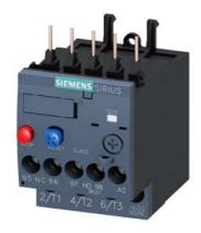
Overload relay 2.2...3.2 A Thermal For motor protection Size S00, Class 10 Contactor mounting Main circuit: Screw Auxiliary circuit: Screw Manual-Automatic-Reset
